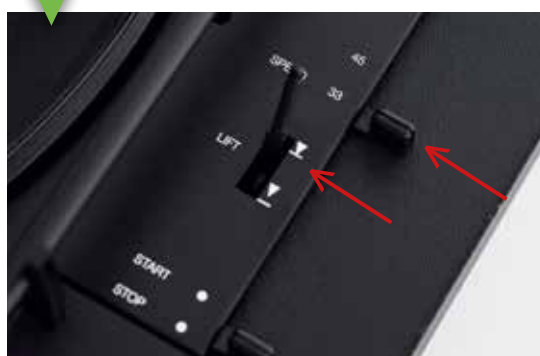
10 Select the playback speed and move the tonearm lift to the upper position.
