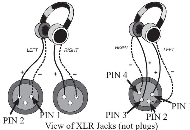
Figure 08– 3-pin XLR wiring    Figure 09– 4-pin XLR wiring
