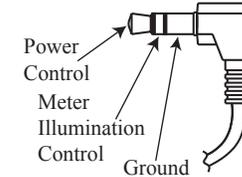
Connect components for Power Control using a 3.5mm stereo mini plug.
