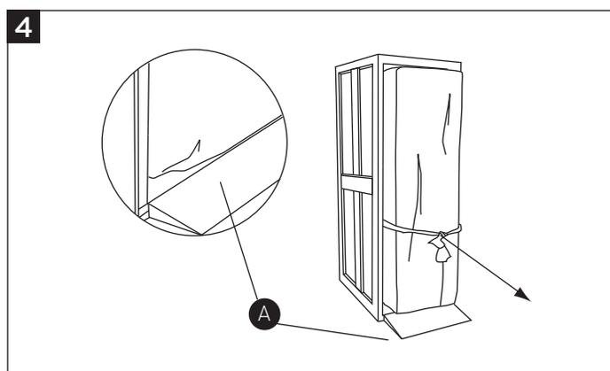
**4 - Install the ramp as indicated. Carefully pull out the loudspeaker thanks to the girth.**
