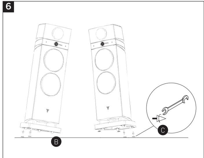
**6 - Once the position is chosen, topple over the loudspeaker on its side (with the protection foams in place) to insert the spikes. You can use counter spikes to protect the floor.**
