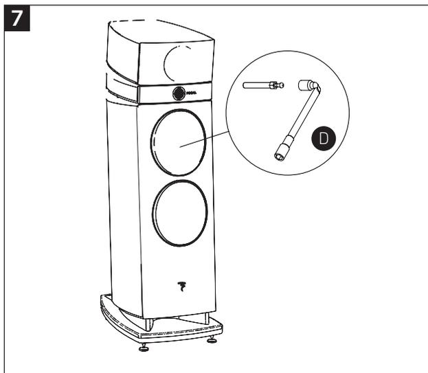
**7 - For safety reasons, screw all the speaker screws (woofer and midrange) that could have been unscrewed during transport. Use the supplied tube wrench.**
