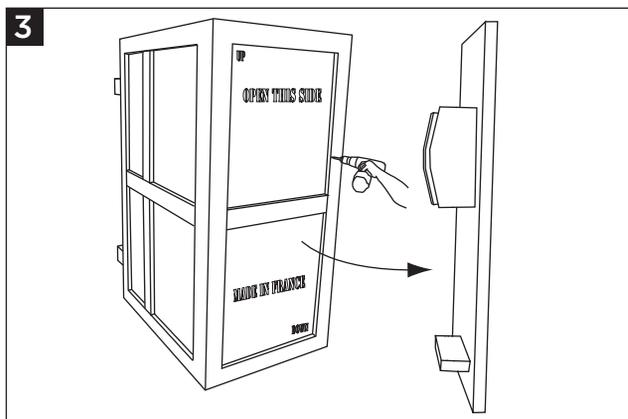
**3 - Unscrew the side panel of the box and remove it.**
