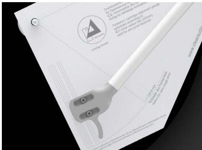
Pic. 10: The tonearm tube must be absolutely parallel
