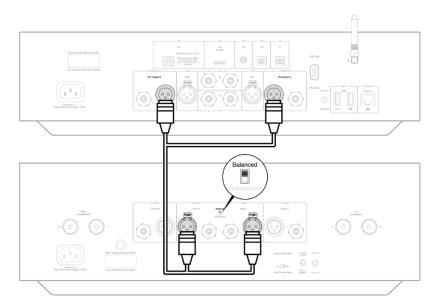
Using XLR cables will enable a balanced analogue connection to your EDGE W. This will provide a cleaner signal path compared to an RCA unbalanced connection, especially over longer cable lengths, however the increase in audio quality they provide is subjective when used over shorter lengths.
