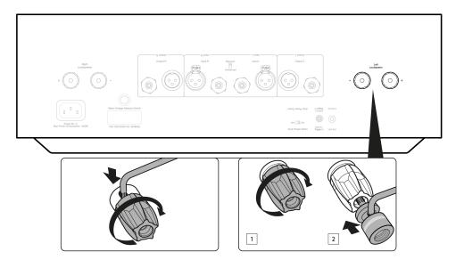
Connect the wires from your left channel loudspeaker to the left positive and negative terminals and the wires from the right channel loudspeaker to the right positive and negative terminals.
