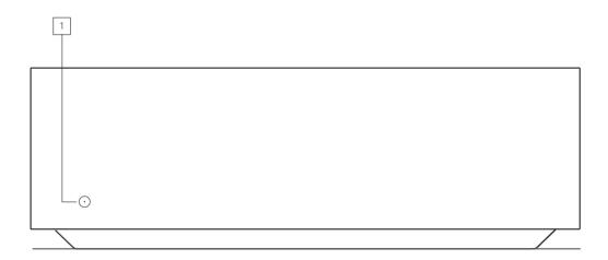
**1. STANDBY/ON** - Switches the unit between Standby mode (indicated by dim LED) and On (indicated by bright LED). Standby mode is a low power mode where the power consumption is less than 0.5 Watts.
