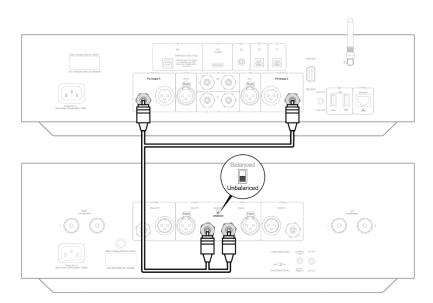
Using RCA cables will enable an unbalanced analogue connection to your EDGE W.
