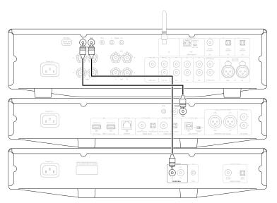
**Note:** The CXA, CXN and CXC all have an Auto Power Down (APD) function. If APD is enabled and one of the devices is switched on but inactive, the device will automatically power down after the selected APD time. This will then switch off all the other connected devices, due to the Control Bus connection.
