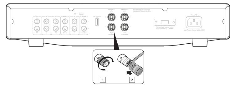
Connect the wires from your left channel loudspeaker to the Left positive and negative terminals and the wires from the right channel loudspeaker to the Right positive and negative terminals.
