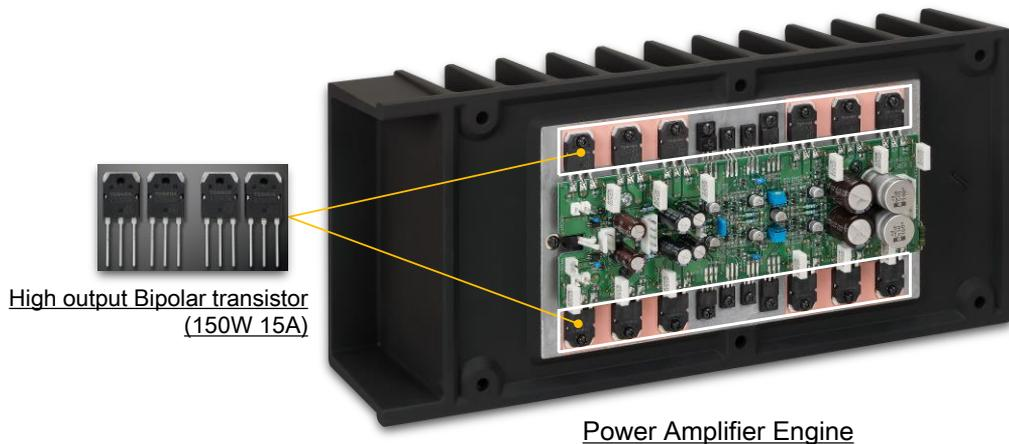
High output Bipolar transistor
