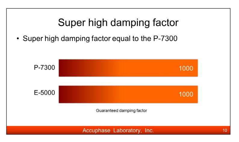
The E-5000 achieves 1000 of guaranteed Damping-Factor, equal to the flagship Class AB stereo power amp P-7300.
