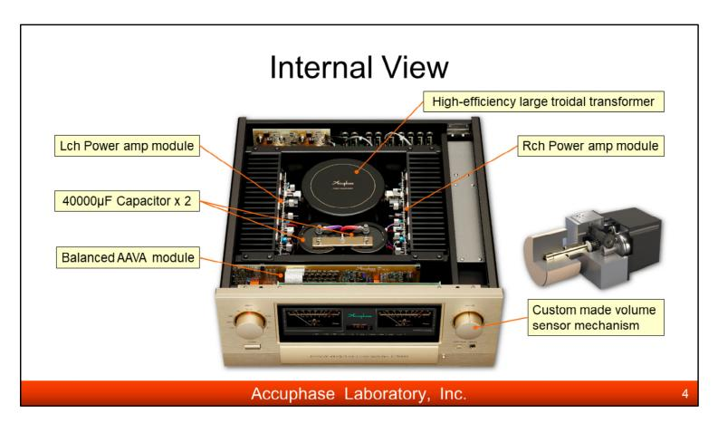
E-5000 has the mono-block construction. The strong power supply with massive, specially-made and high-efficiency toroidal transformer and 40000µF filtering capacitors are installed in the center of the unit. In addition, the two power amplifier modules are kept separate for the left and right channels.
