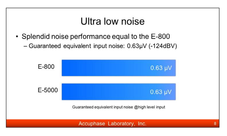
The E-5000 realizes -124dB (  $0.63\mu V$  ) of equivalent input noise equal to the flagship class-A integrated amp E-800.
