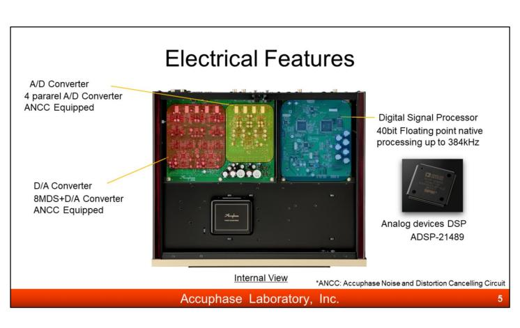
DG-68 has the digital signal processing modules on the right side, and the mixed-signal processors including A/D, D/A converter on the left.
