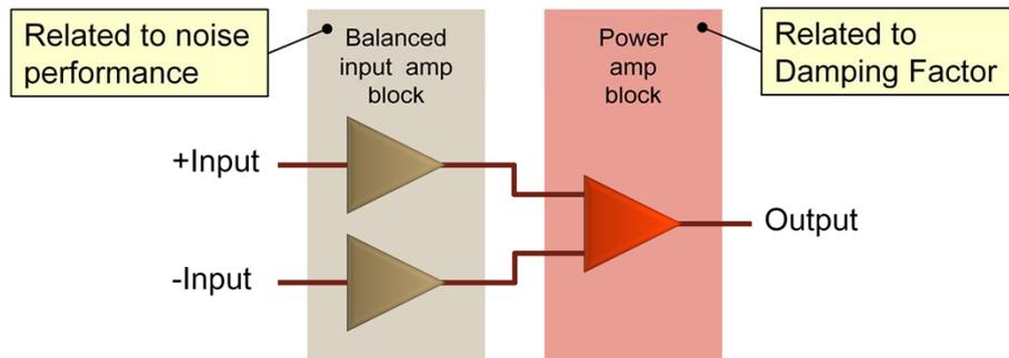
A-250 Instrumentation amplifier configuration
