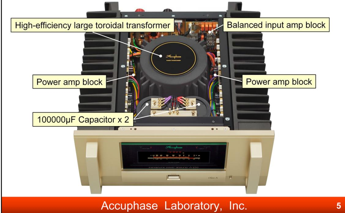
Strong power supply with a massive high-efficiency Toroidal transformer and two large 100000µF filtering capacitors are installed.
